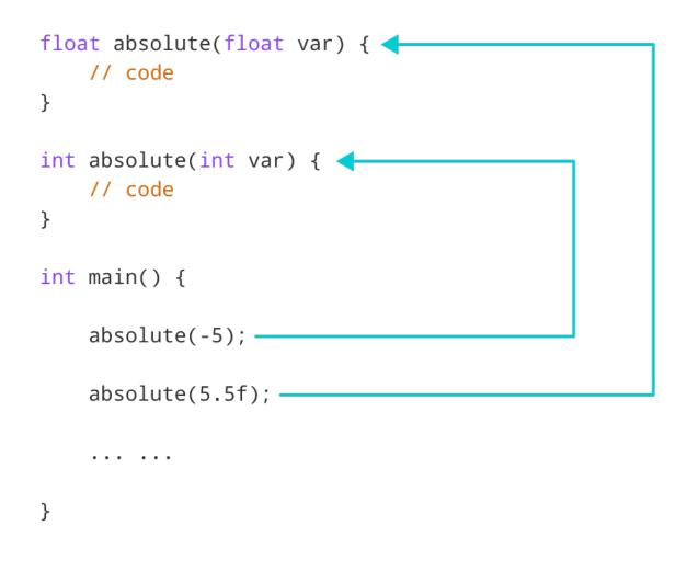
Working of overloading for the absolute() function
