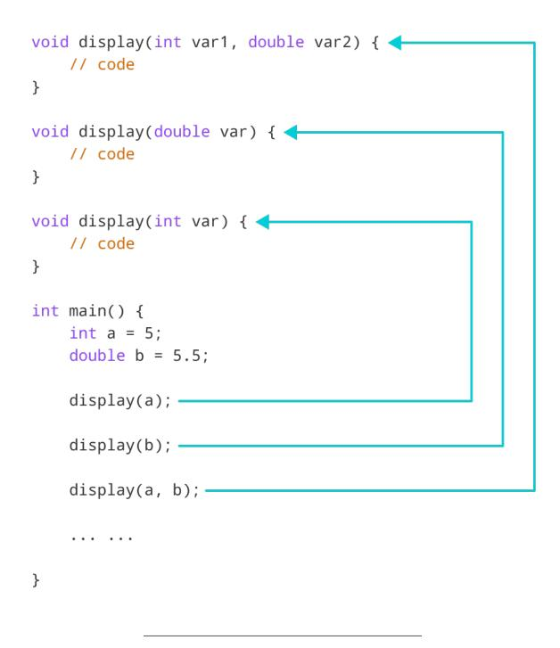
Working of overloading for the display() function
